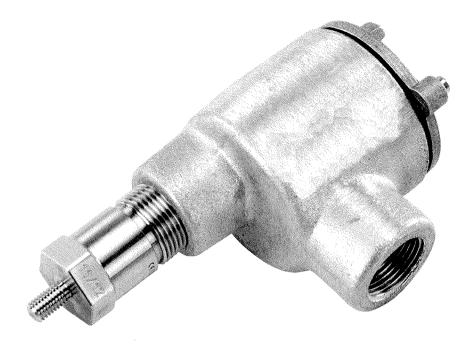
This transmitter can provide an electrical signal directly proportional to the vibration of the point to which it is fastened, with direct interface to an acquisition system made in 2-wire technique (4-20 mA current loop).
